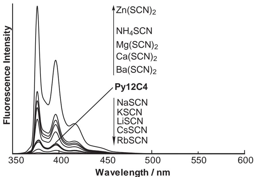
Fig. 3. Fluorescence spectra of **2** ( $2.0 \times 10^{-6}$  M) with and without various guest cations ( $1.0 \times 10^{-2}$  M) in  $\text{CH}_3\text{OH}-\text{CHCl}_3$  (9 : 1 v/v) at room temperature.
