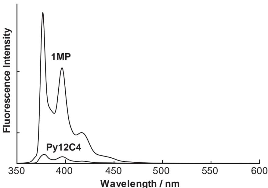
Fig. 2. Fluorescence spectra of **Py12C4** ( $2.0 \times 10^{-6}$  M) and 1-methylpyrene (**1MP**,  $2.0 \times 10^{-6}$  M) in  $\text{CH}_3\text{OH}-\text{CHCl}_3$  (9 : 1 v/v) at room temperature, as excited at 343 nm.
