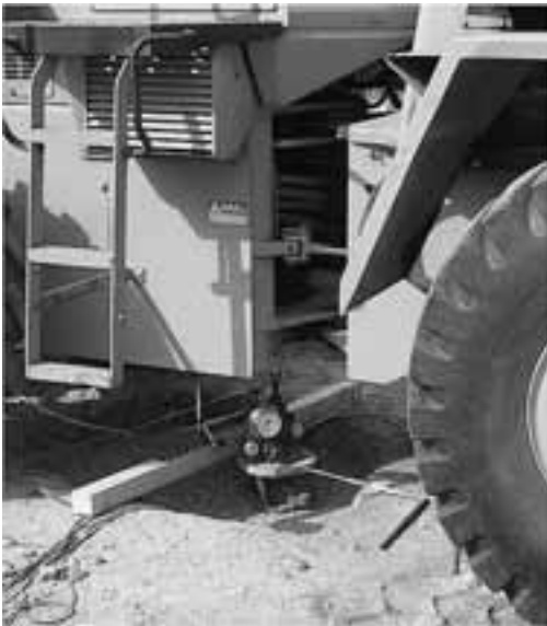
Figure 2 Plate Bearing Test
